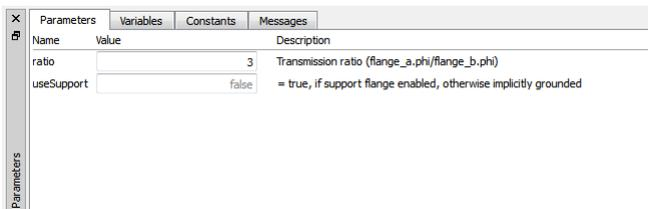
**Figure 3-11:** Editing the transmission ratio of an ideal gear component in the *Model Center*.
