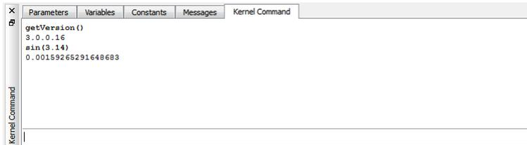
**Figure 3-71:** Executing commands in the **Kernel Command** view.
