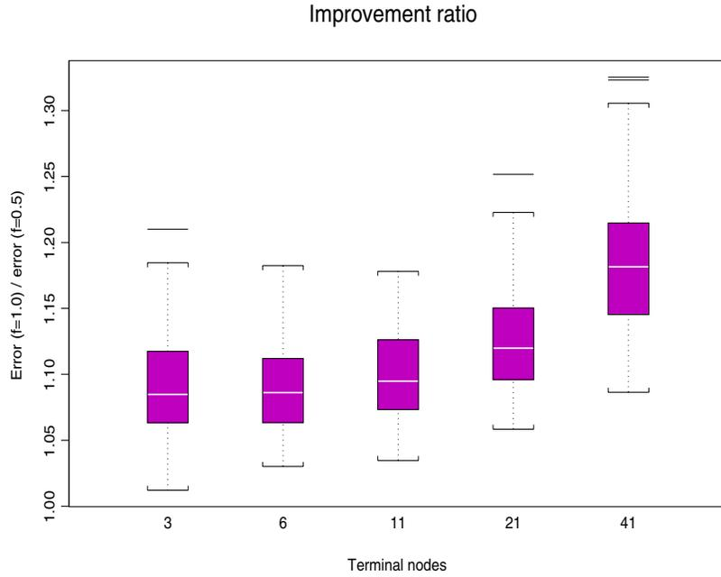
Figure 4: Distributions of the ratio of the error of the deterministic algorithm to that using 50% sampling with different sized regression trees as base learner, for small ( $N = 500$ ) training samples.
