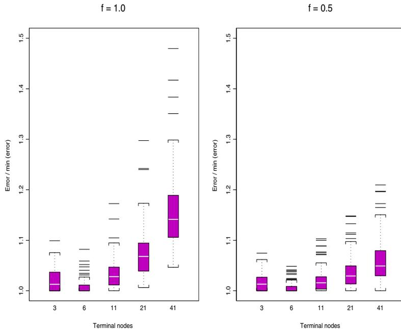
Figure 3: Distributions of absolute approximation error, relative to the best, for different sized regression trees as base learner, for small ( $N = 500$ ) training samples. The left panel is for training on the full sample. The right panel is with 50% random subsampling at each iteration.
